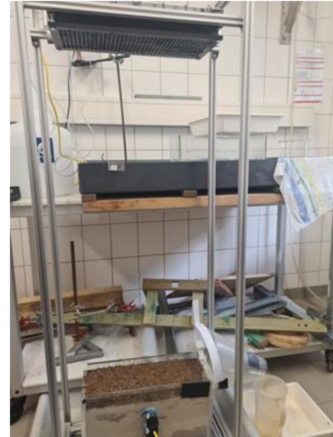
Self designed setup for the determination of dust emission and water erosion
